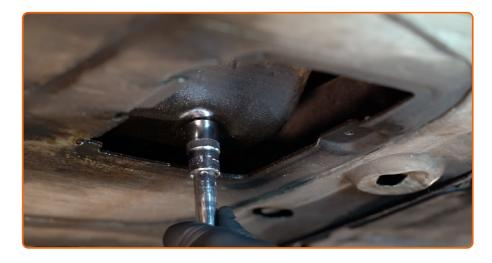
Unscrew the drain plug. Use a drive socket #17. Use a ratchet wrench.
