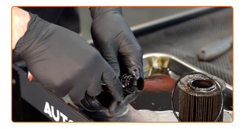
Remove old o-rings from the oil filter cover. Use a flat screwdriver.
