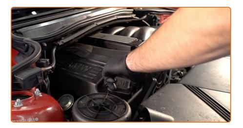
Tighten the oil filler cap.
