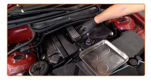
Screw the new filter into its place.
