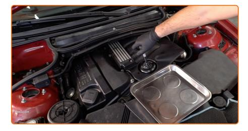
Unscrew the oil filter. Use the 86/16 F socket.
