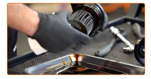
Detach the oil filter from the filter cover.
