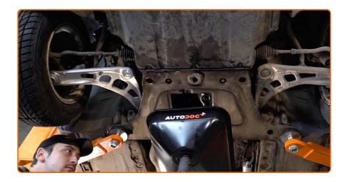
Put a waste oil container with at least 6 I capacity under the drainage hole.
