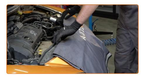
Remove the fender protection cover.
