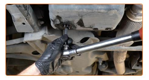
Screw in the new drainage plug and tighten it. Use HEX No.H6. Use a torque wrench. Tighten it to 30 Nm torque.
