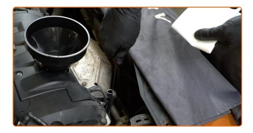
Check the oil level using the dipstick. Top up oil if necessary.
