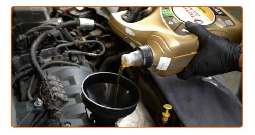
Pour oil into the engine through the filler. Required amount of oil: 3 L.
