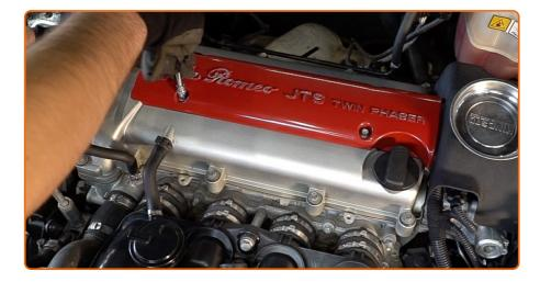
Undo the engine cover screws (4 pieces). Use a drive socket #8. Use a ratchet wrench.
