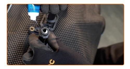
Treat the mounting seats of the spark plugs on the ignition coil. Use high-temperature grease.
