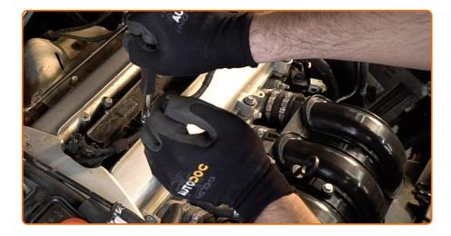
Unscrew the ignition coil bracket. Use a drive socket #10. Use a ratchet wrench.
