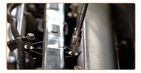
Tighten the ignition coil fastening. Use a drive socket #10. Use a torque wrench. Tighten it to 8 nm torque.
