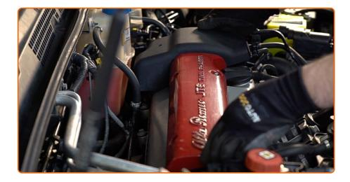
Install the engine cover and secure it. Use a drive socket #8. Use a ratchet wrench.
