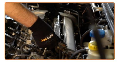
Install the ignition coil to the spark plug well. Make sure you hear a click indicating that it is locked in place.
