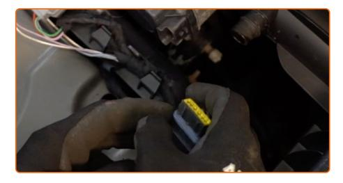
Detach the throttle valve connectors.
