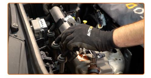
Pry up the ignition coil. Take out the ignition coil from the spark plug well.
