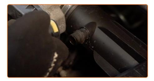
Disconnect the crankcase ventilation hose from the air duct.
