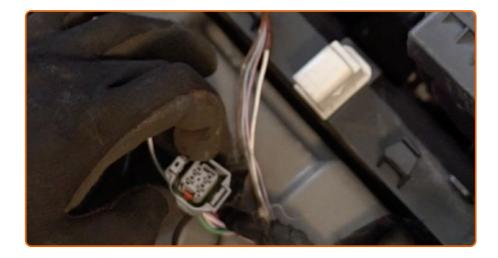
Detach the connector from the ignition coil.
