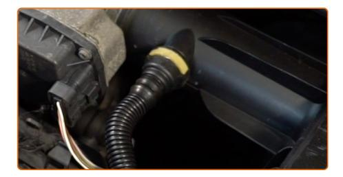
Remove the microfibre cloth from the PCV valve hole.
