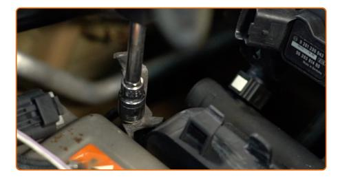
Tighten the ignition coil fastening. Use a drive socket #10. Use a torque wrench. Tighten it to 9 nm torque.
