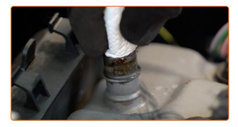
Cover the PCV valve hole with a microfibre cloth to prevent dirt and foreign objects from getting into the system.
