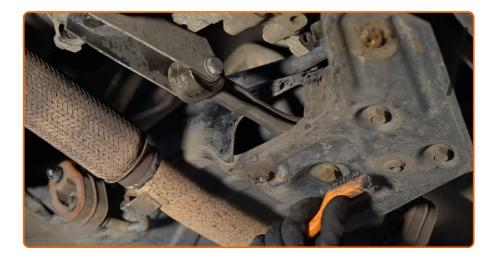
Clean the engine mount fasteners. Use a wire brush. Use WD-40 spray.
