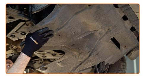
Remove the lower sound insulation.
