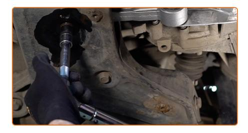
Use a drive socket #16. Use a torque wrench. Tighten it to 57 Nm torque.
