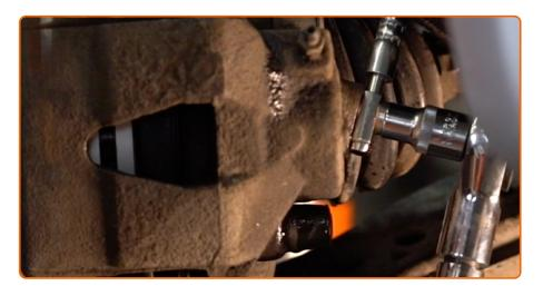
Tighten the fastener connecting the brake pipe to the brake caliper. Use a drive socket #11. Use a torque wrench. Tighten it to 18 Nm torque.
