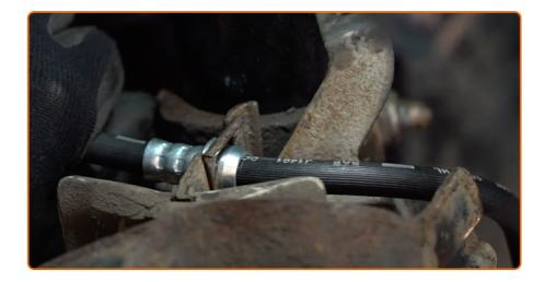
Install the brake hose retaining clip. Use a rubber mallet.
