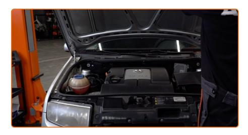
Open the bonnet. Unscrew the brake fluid reservoir cap.
