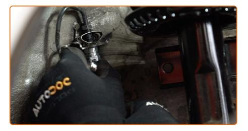
Screw the brake hose onto the brake circuit pipe. Use a combination spanner #11. Use a torque wrench. Tighten it to 15 Nm torque.
