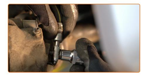
Unscrew the brake hose from the brake caliper. Use a drive socket #11. Use a ratchet wrench.
