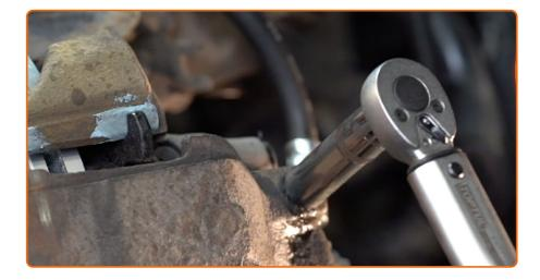
Tighten the brake caliper bleed screw. Use a drive socket #11. Use a torque wrench. Tighten it to 13 Nm torque.
