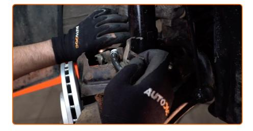
Fasten the brake hose on the strut.
